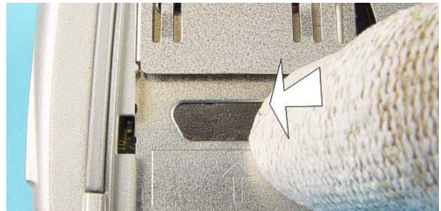
6.) Put back the Sealing Tape after the flashing procedure.
